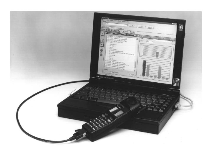
The Agilent Technologies E7460A service quality analysis system is used to obtain call performance data versus location to assess the service coverage of wireless communications networks using IS-95 and J-STD-008 CDMA technologies. A PC interfaces to a CDMA mobile phone. Each system includes PC software, a PCMCIA serial port card to connect the phone to the PC. The system can be integrated with a GPS receiver and mapping software.
